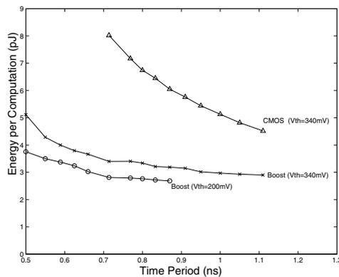
**Figure 7. Energy consumption vs frequency for 8-bit multipliers**
