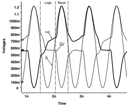
Figure 3. SPICE waveforms of a Boost Logic inverter
