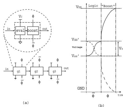
Figure 1. Boost Logic (a) Cascade and (b) Operation
