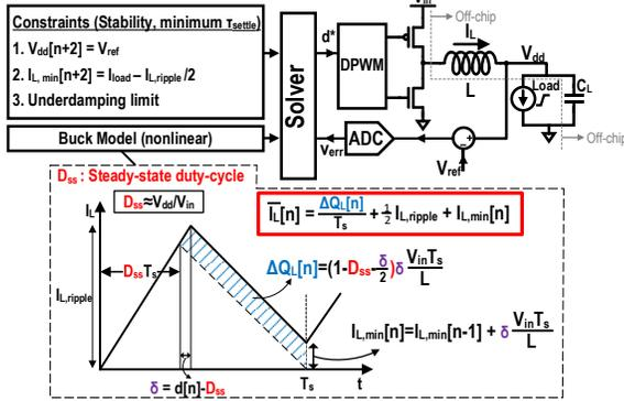
Fig.1: MPC Architecture and non-linear buck model used by Solver.
