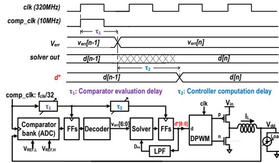
Fig. 6: MPC Test chip architecture. Delayed clocks provide time for Comparator and Solver evaluation with glitch-free operation.
