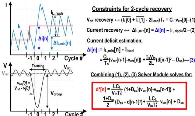
Fig.2: MPC Constraint Equations of  $d^*[n]$  for 2-cycle  $V_{dd}$  restoration.
