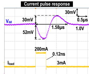
Fig. 9: Measured MPC  $V_{dd}$  response to  $I_{load}$  pulse with step-down occurring during  $\tau_{settle}$ .
