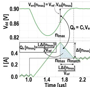
Fig. 3: Stable MPC response under  $d[n]$  saturation through  $Q_s$  tracking.
