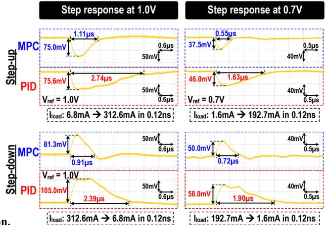
Fig. 7: Measured  $V_{dd}$  response to a load-step for MPC and optimally tuned PID controllers. Both incur  $d[n]$  saturation resulting in similar  $V_{droop}$ .
