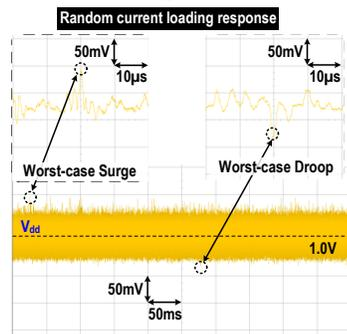
Fig. 8: Measured MPC  $V_{dd}$  waveforms under random loading conditions.
