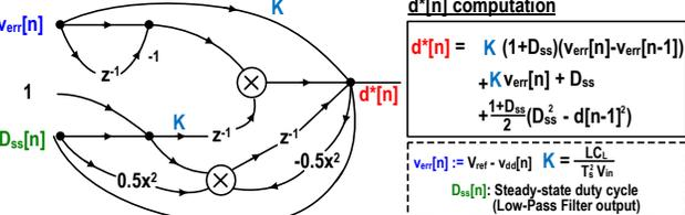
Fig. 5: Dataflow graph for  $d^*[n]$  computation.
